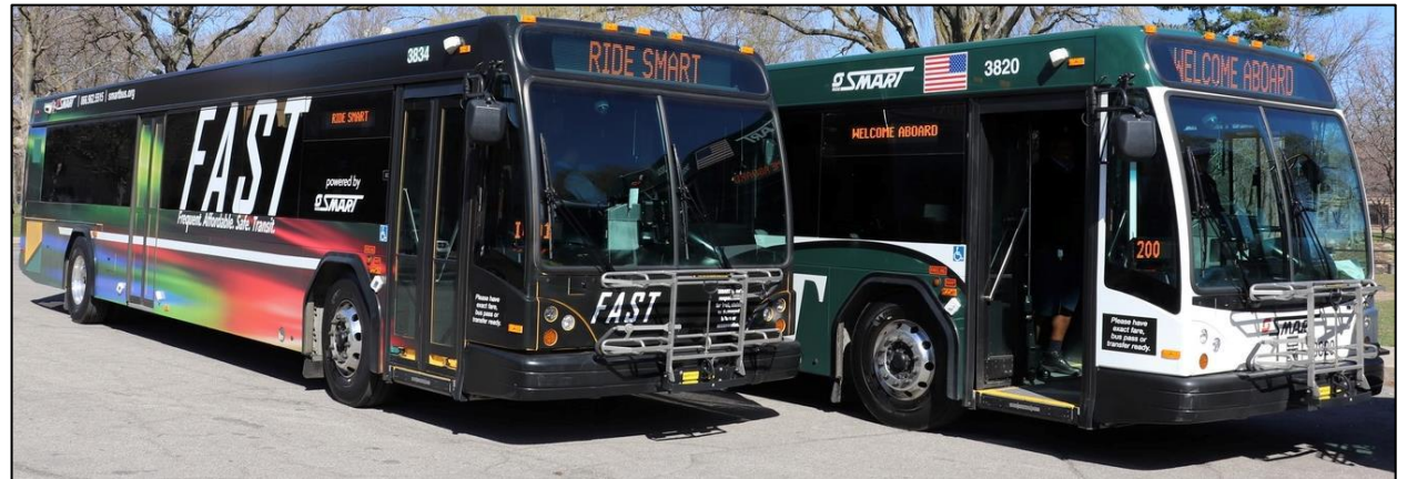
Image: 40-foot SMART buses. Articulated buses are 60 feet in length. Weight ranges from 25,000-70,000 pounds.
