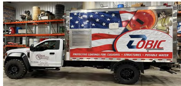
Figure 12. ART's offroad installation truck built specifically for applications with difficult access.
