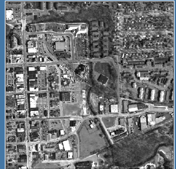
The Paint Creek in the City of Rochester was straightened and re-routed near its confluence with the Clinton River, allowing the development of the municipal library along the banks.
