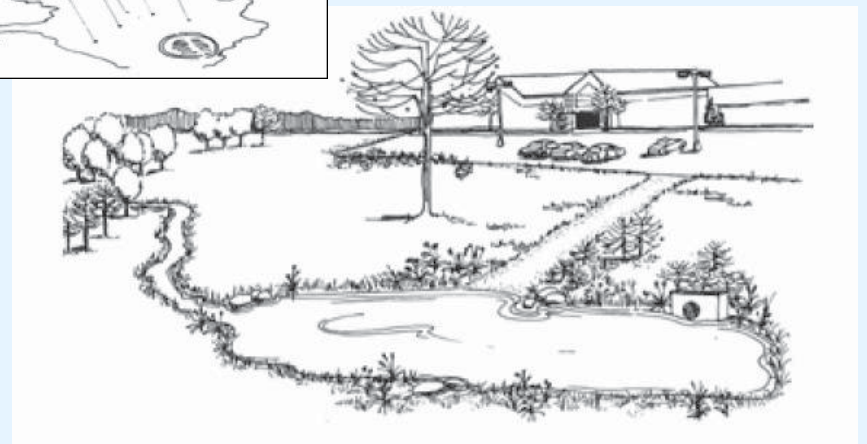
Alternative Stormwater Conveyance System (Photo Credit: Carlisle/Wortman Associates, Inc.)
