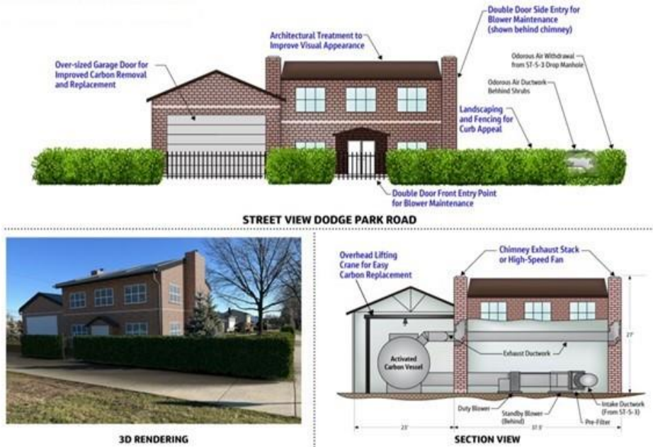
Preferred Alternative at ST-S-3: Odor control equipment located inside of a replica house
